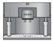
The bottom of the funnel fits into the drip tray to enable the descaling agent to be collected in it.
